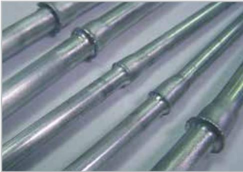
Replacing torch brazing of aluminum tubing to air conditioning evaporator. Using flux cored aluminum braze rings and a split helix induction coil for easy access to the joint area. 5 kW at 260 kHz for 12 seconds to 565°C (1050°F).
