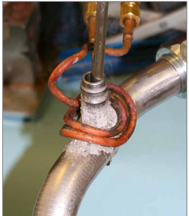
Brazing steel tube fittings used on trucks. 300 kHz at 3 kW for 45 seconds to 732°C (1350°F).
