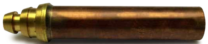
Induction brazing a brass mixing nozzle onto a twin feed copper tube for an oxyacetylene torch nozzle assembly. 6 kW at 380 kHz for 36 seconds to 732°C (1350°F).
