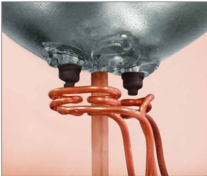
Replacing torch brazing with a multi-position helical coil to induction braze two or three nickel plated steel ferrules to nickel plated pins from an automobile light bulb. 8 kW at 360 kHz for 6 seconds to 620°C (1150°F).
