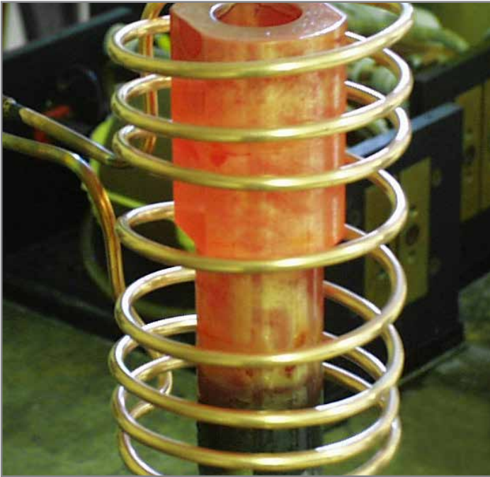
Induction brazing is an excellent method of joining parts made of dissimilar metals. Applications with mixed metal joining include steel-to-copper, steel-to-brass and brass-to-copper. With these materials, it's all about timing.
