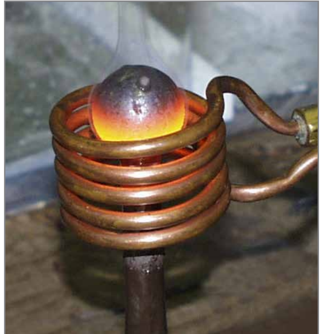
Steel to steel brazing of part of a regulator used in the oil industry. 200 kHz at 8 kW for 9 seconds to 732°C (1350°F).
