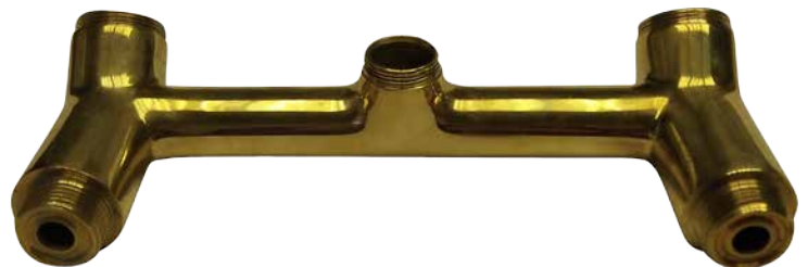
Replacing torch brazing for two brass joints on a faucet manifold. Each joint was induction brazed using a saddle coil. 22 kW at 90 kHz for 30 seconds to 620°C (1150°F).
