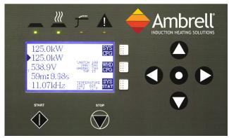
**EKOHEAT** features a front panel programmable controller for monitoring, timer and power-level control, diagnostics and system configuration. Up to 10 ten-step heating profiles can be configured to control power levels over your specified timing requirements.
