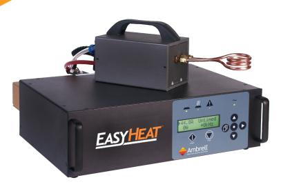
The compact EASYHEAT Air is an air-cooled induction heating system that offers peak power of 2 kW. It is a reliable solution for heating parts with a quick, clean source of heat. With a movable work head that can be located up to 3m (10') from the power supply, it is ideal for repeatable, non-contact heating of parts.
