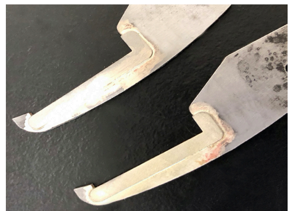
Figure 11: Flat carbides to steel brazed using induction heating.
