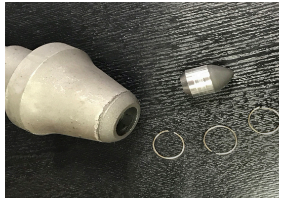
Figure 7: Carbide and steel parts along with three braze wire preforms.
