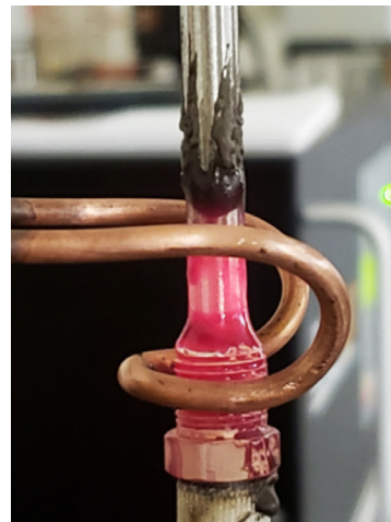
Figure 3: Open "U" shaped induction coil heating a steel tube and brass fitting for brazing.
