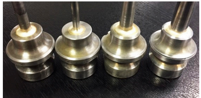
Figure 13: Finished brazed samples with minimal runoff of the braze to the outer diameter of the part.
