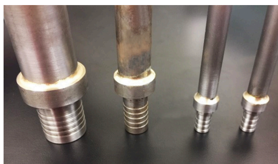
Figure 16: Braze joint between steel tube and brass fitting. The joints would benefit from a braze stop off in the brass threads to prevent the overflow of braze alloy.
