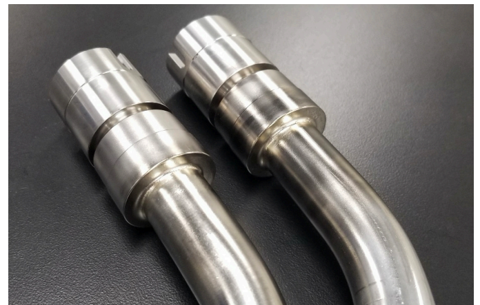
Figure 5: Stainless parts that are induction brazed.
