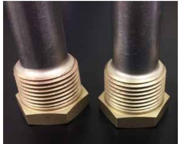
Figure 18: Braze joint between steel tube and brass fitting. The joints would benefit from a braze stop off in the brass threads to prevent the overflow of braze alloy.
