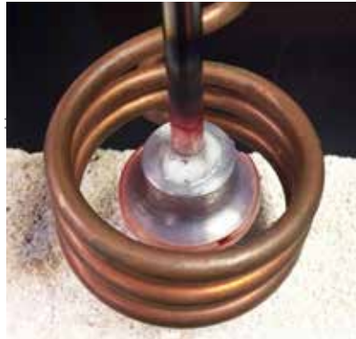
Figure 12: Heating of steel assemblies with white flux at the joint, shielding the braze wire pre-form and the part.
