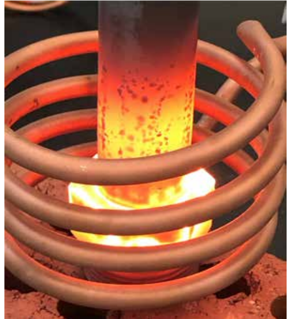
Figure 21: Oxidation of steel parts when heated to 1900-2000 °F (1037-1093 °C) in air. An inert atmosphere is required to prevent this oxidation and facilitate the flow of the braze alloy.
