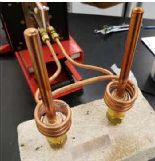
Figure 2: Two parts heated in a water-cooled copper induction coil.
