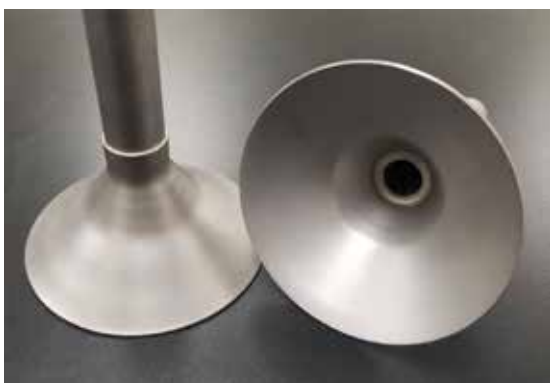
Figure 4: Flow of braze alloy all around the circumference of the joint due to capillary action.
