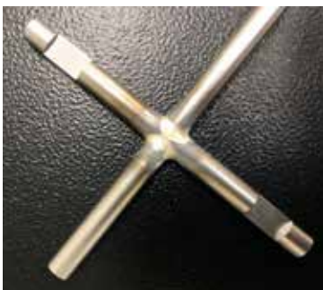
Figure 15: Braze joint between two steel rods. The fillet is an easy visual indication of the braze flow.
