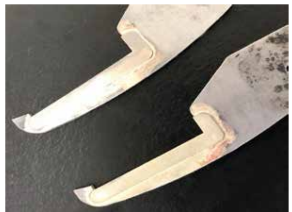
Figure 11: Flat carbides to steel brazed using induction heating.
