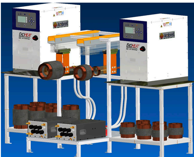
Figure 12: Induction heating of steel stator using an ID coil. One induction coil that oscillates back and forth is used to heat various diameter and length parts.
