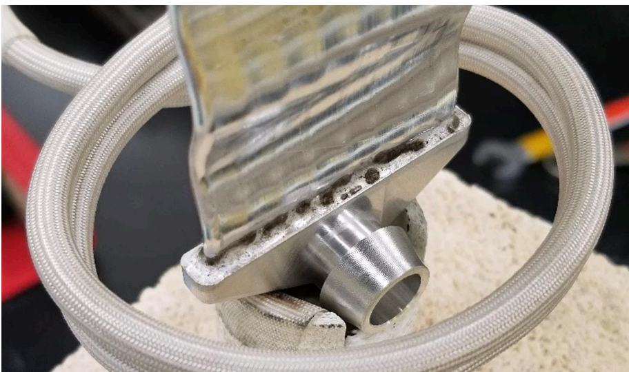
Figure 24: Finished Induction braze joint on an aluminum assembly. Braze alloy has flowed well, wetting all surfaces.
