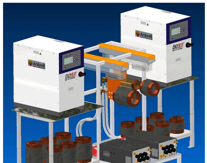
Figure 13: Induction heating of steel stator using an ID coil. The setup allows for different diameter and length parts to be run on the same station without changeover concerns.
