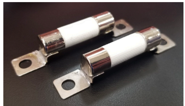
Figure 21: Induction soldering of the tabs on fuses. Typical cycle is 3-4 seconds.
