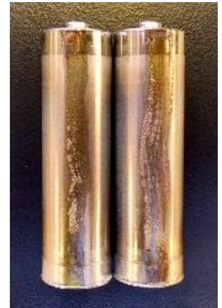
Figure 20: Battery shells after passing through a channel type induction coil. Paint turns clear when parts reach temperature.
