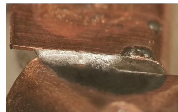
Figure 22: Close-up of good solder flow in a copper-to-copper joint inside a fuse with induction.
