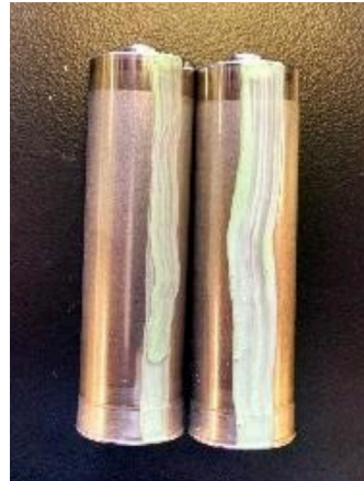
Figure 18: Battery casings with 400 °F temperature paint before heat testing.
