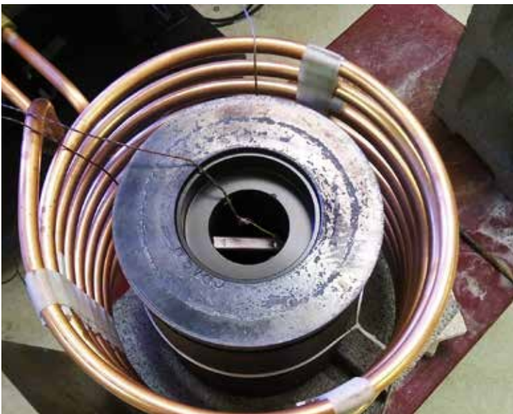
Figure 8: Heating of 6-inch diameter steel rotor using an OD coil.
