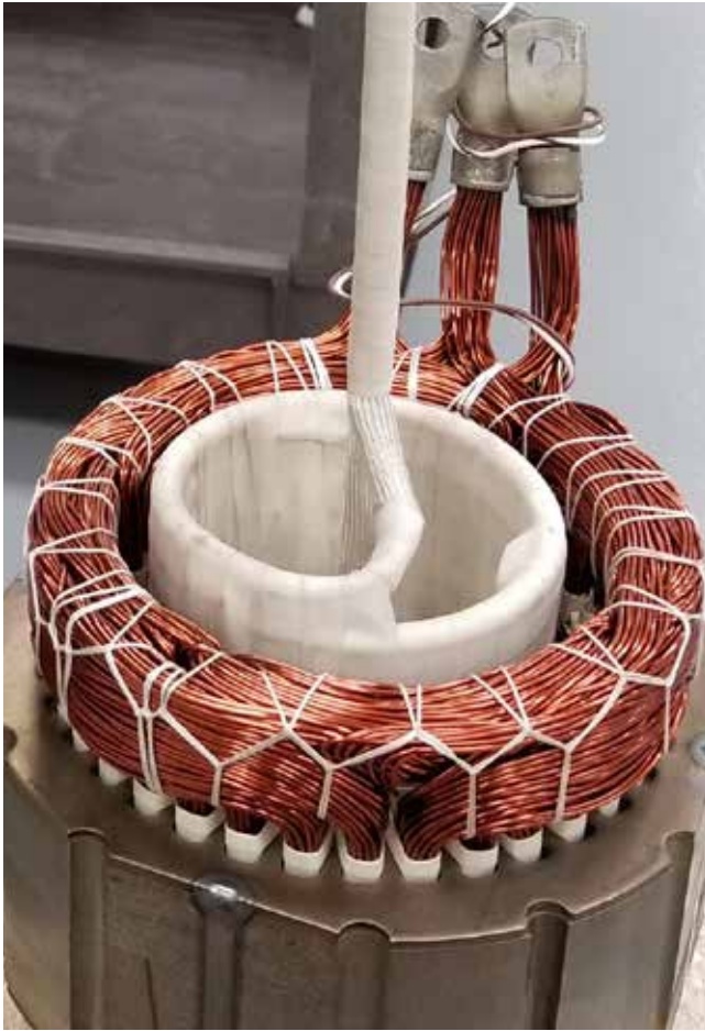
Figure 11: ID coil to heat a steel stator with copper wires before a varnish dripping process.
