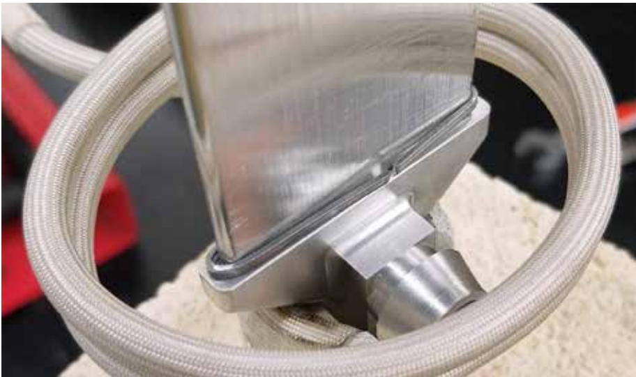
Figure 23: Aluminum induction brazing setup for the cooling channel to end fitting.
