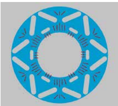
Figure 4: Heat transfer through the steel laminations of a steel rotor with ID heating.
