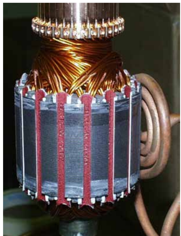
Figure 17: Pancake style coil for preheating a steel rotor.
