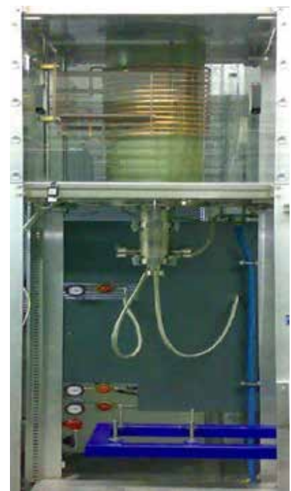
Figure 28: PVT crystal growth setup using induction.
