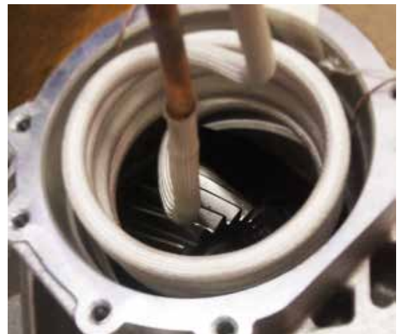
Figure 2: Induction heating coil setup for heating aluminum assembly for a shrink fitting application.
