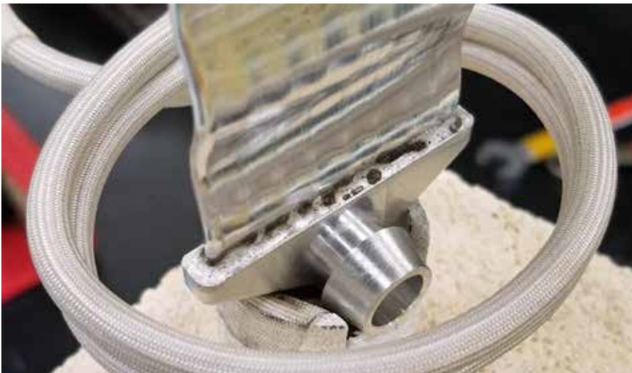
Figure 24: Finished Induction braze joint on an aluminum assembly. Braze alloy has flowed well, wetting all surfaces.
