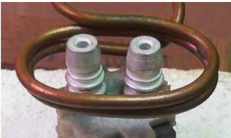
The assembly inside the coil prior to heating.
