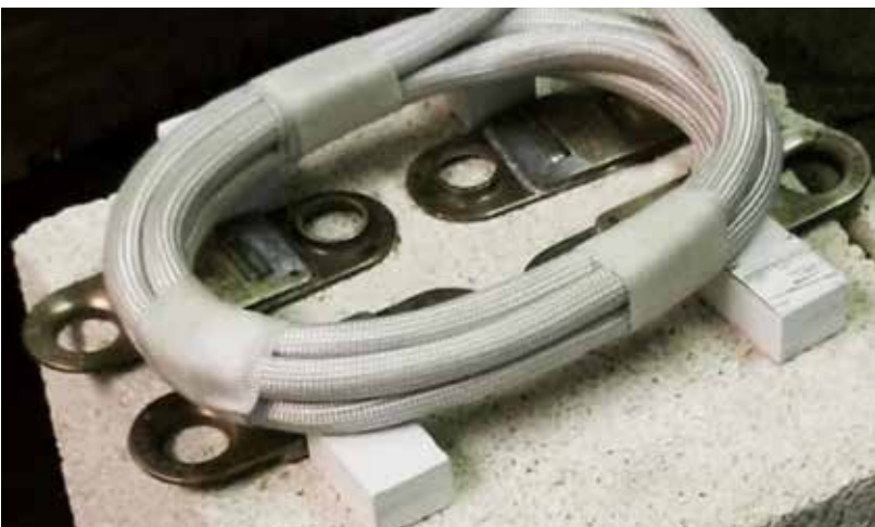
Four copper strips being heated concurrently with an induction coil.
