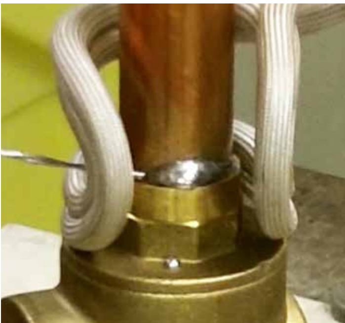
The assembly inside the induction heating coil during soldering.
