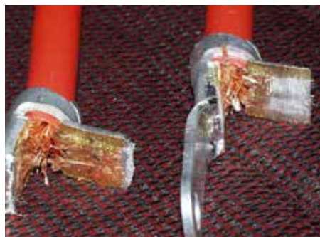
The part on the right was done by the EASYHEAT, and the part on the left was done by the previous induction heating system – the penetration of the solder is superior on the right.
