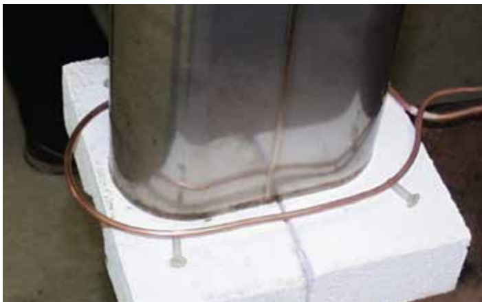
Canister is staged within single-turn coil; solder flows in the cavity formed with the steel end-plate.
