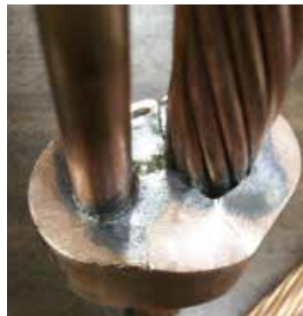
The joint made during the vertical orientation.
