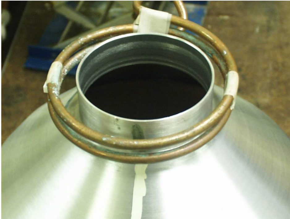
Temperature indicating paint shows the 1” heat zone annealed on the cryogenic dewar
