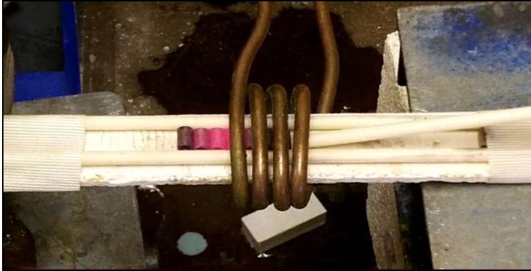
The tubes in the ramp being heated via the induction coil
