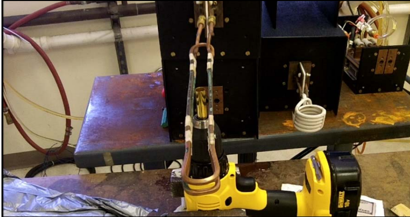
The test set up, with the ammunition casing in a rotating device.
