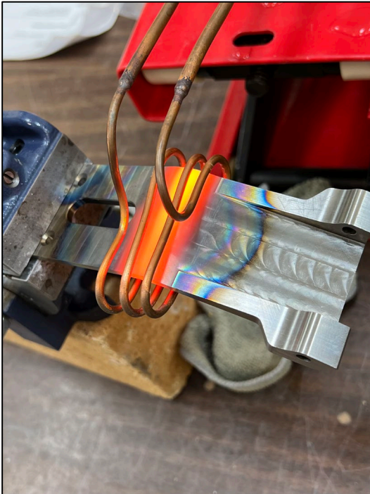
The part inside the coil during heating.
