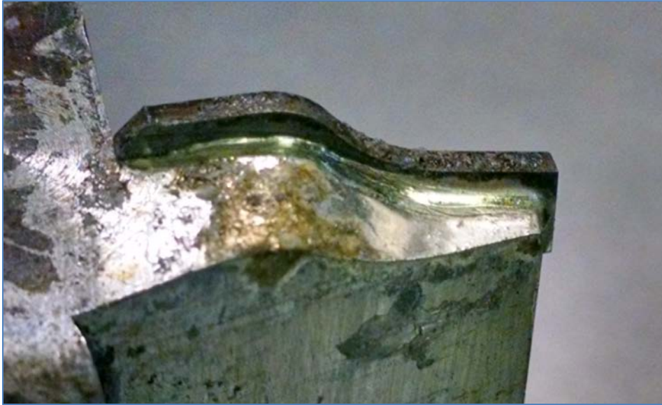
Test material: steel cutting bit with diamond-carbide insert
