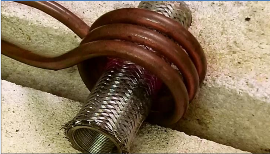
The magnetic steel tube at temperature showing a dull red glow.
