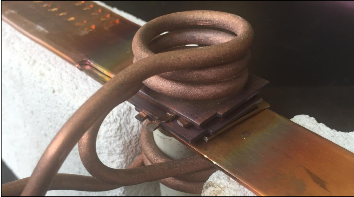
The copper strip assembly inside the multi-turn split helical coil.
