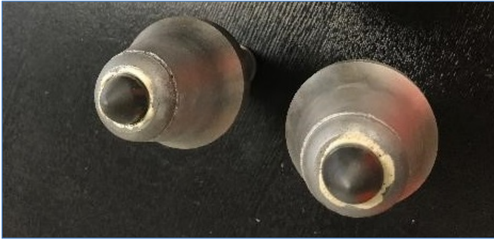
Two steel and carbide assemblies after brazing.
