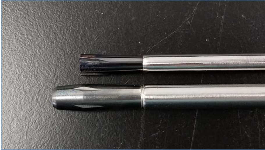
Two steel and carbide assemblies after brazing.
