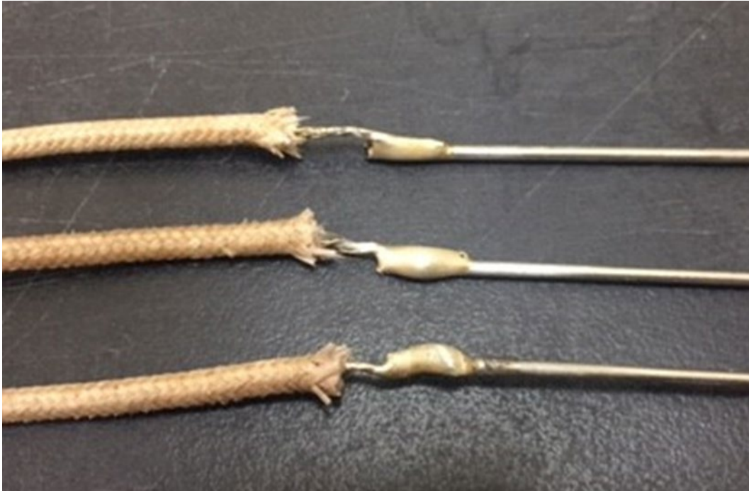
The brazed joints from this application.
