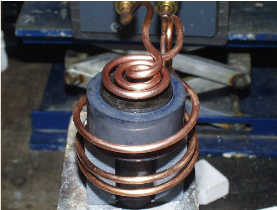
A combination pancake/helical coil is used for easy loading and unloading of the part.
