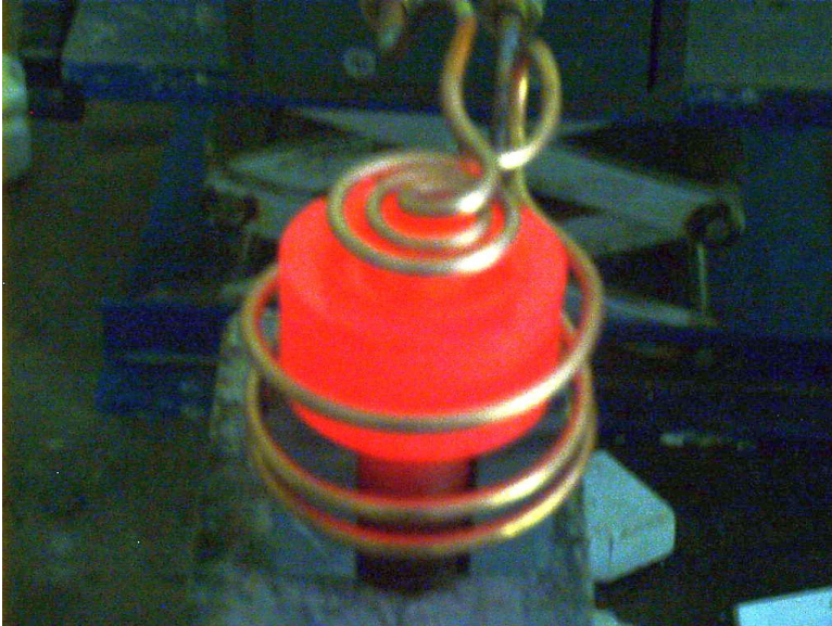
The heat pattern on the assembly illustrates even distribution of heat.
