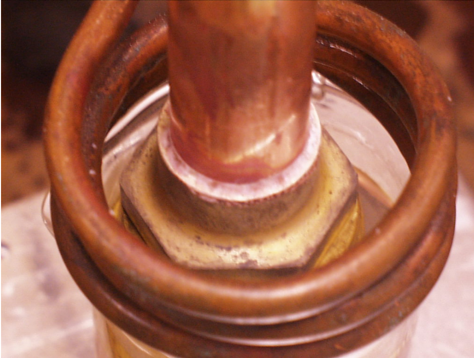
Brass fitting partially submerged in water bath
