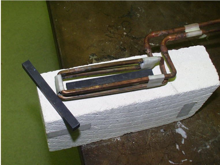
Coil and two pieces of graphite used to heat steel assembly
