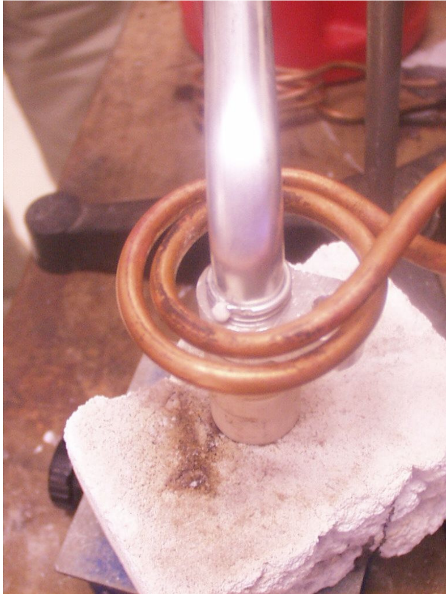
Coil in position for brazing joint
