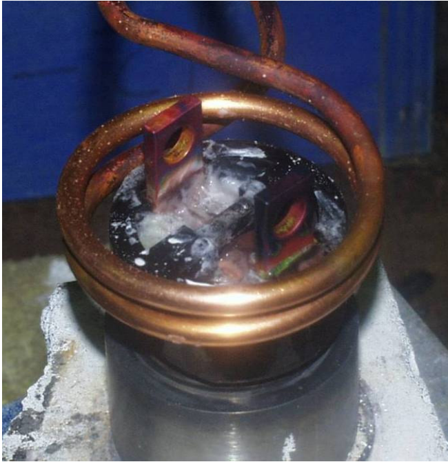
Heater connector assembly in coil heating for brazing application
