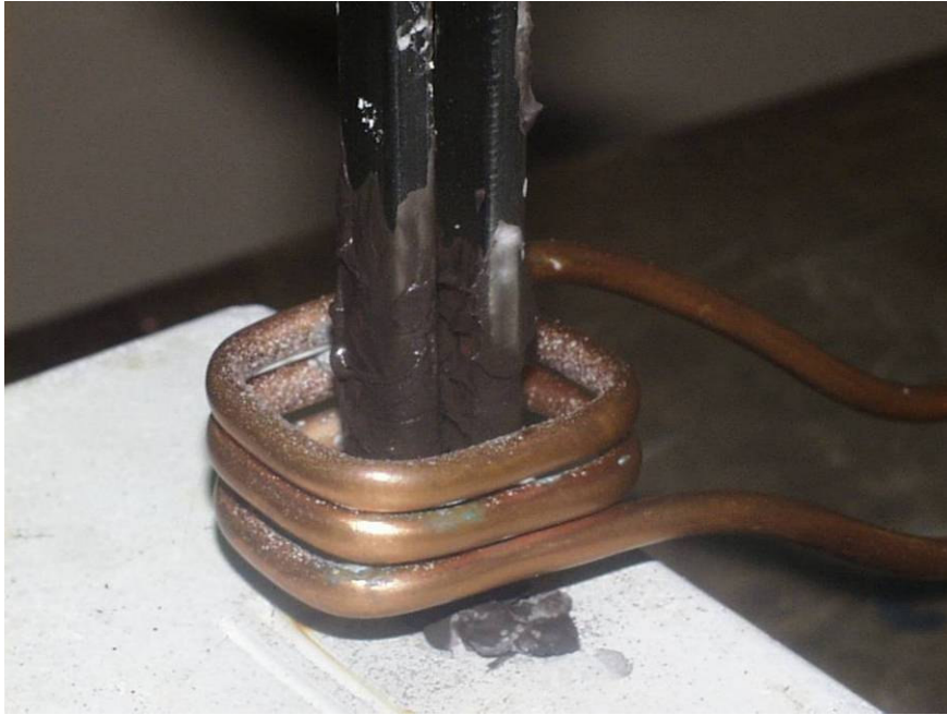
End plug and grill in place for brazing application
