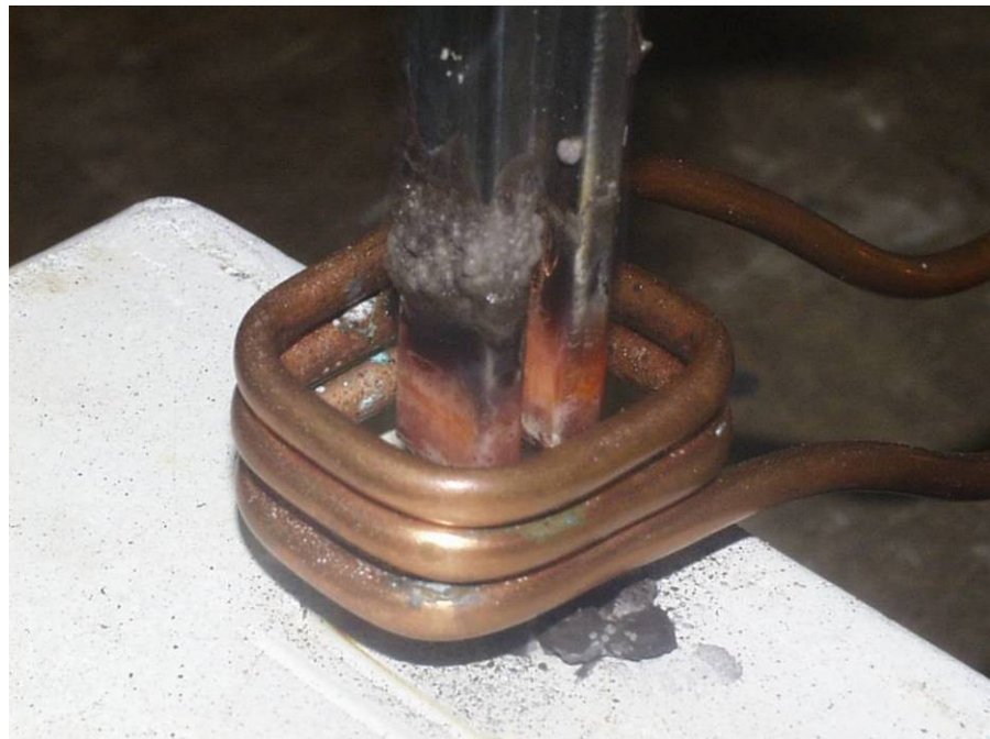
After 30 seconds the braze flows to create joint
