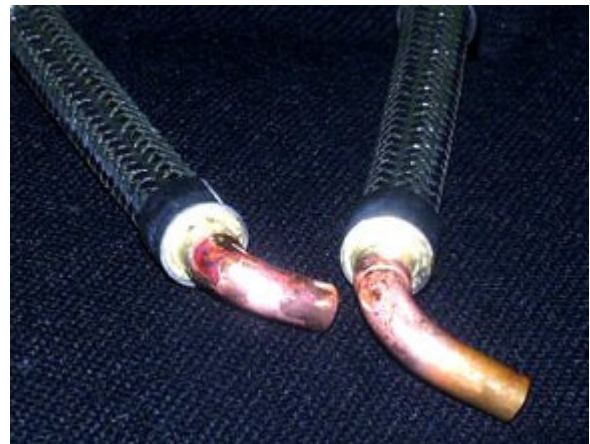
Finished brazed hose and copper assembly
