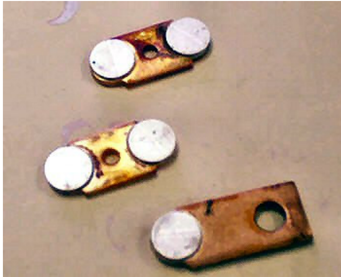
Finished brazed contacts and bus
