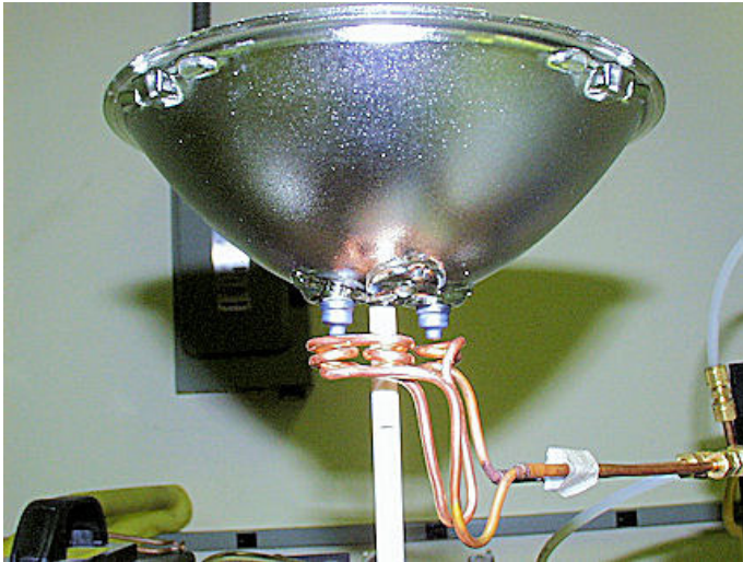
Underside of light bulb with leads in the ferrules
