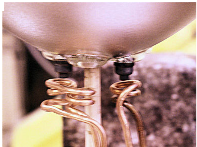
Close up of coil placement
