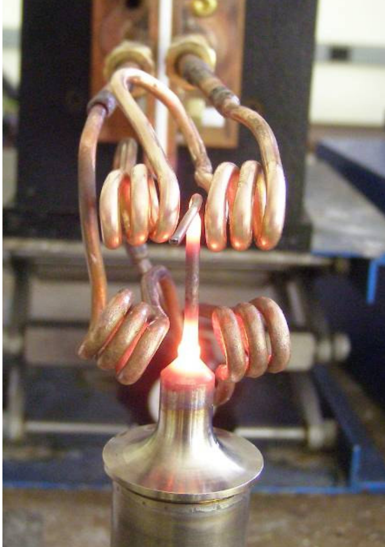
The two braze locations are heated simultaneously
