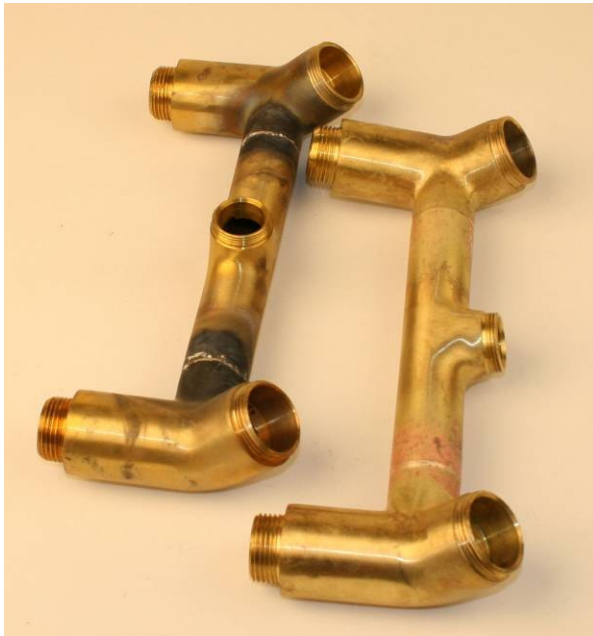
Completed brazed assembly, assembly on right brazed with induction, left assembly by flame
