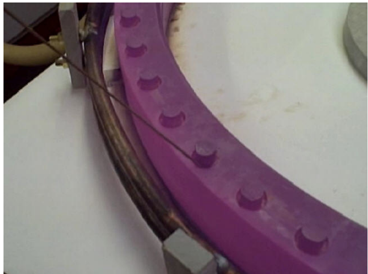
Slip ring at temperature ready for brazing the vertical bars
