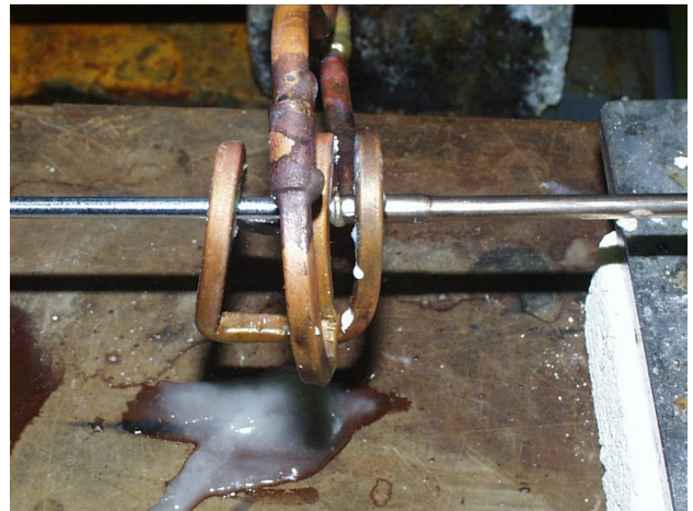
Steel to steel horizontal joint
