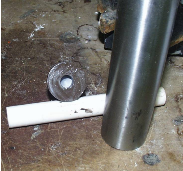
Bottom of carbide (showing countersunk hole) and shaft
