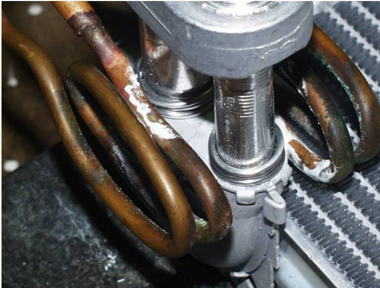
Assembly in coil prior to brazing showing the 3 braze rings in place
