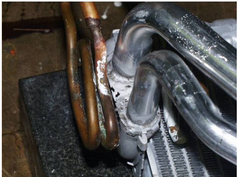
Power has been applied and the braze rings have melted creating an air tight braze
