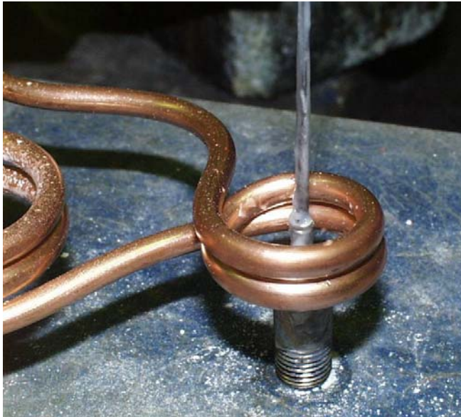
0.188" (4.8mm) OD probe in smaller diameter coil for brazing
