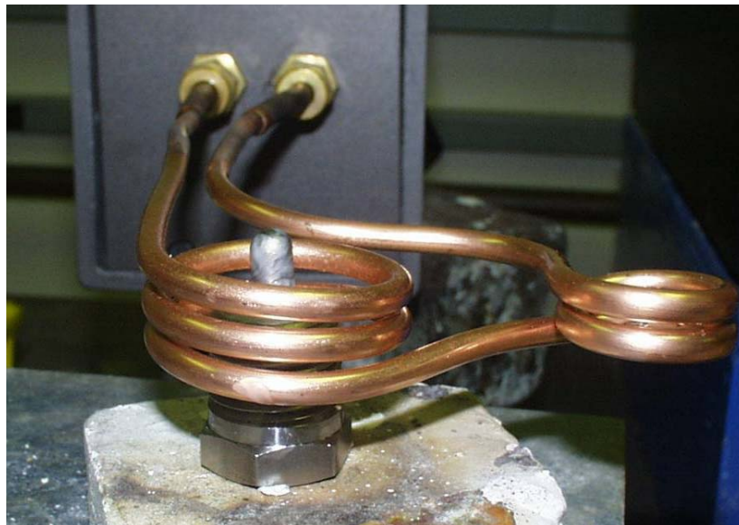
0.25" (6.4mm) OD probe in larger diameter coil for brazing
