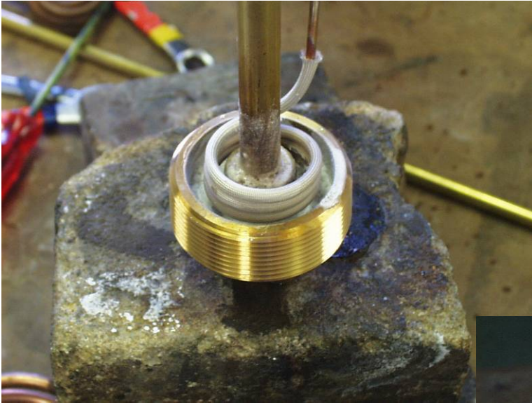
Smaller steel tube and end plug assembly being brazed
