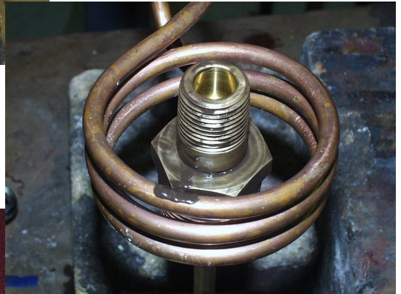
Larger steel end plug prior to brazing
