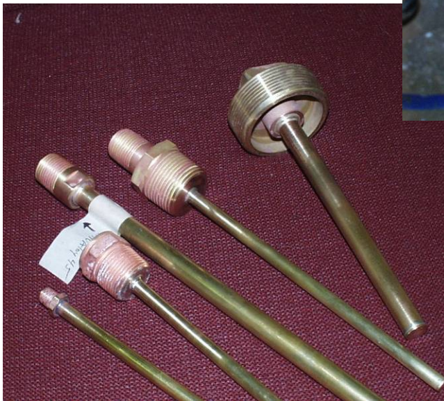
Multiple steel and brass assemblies brazed in this application
