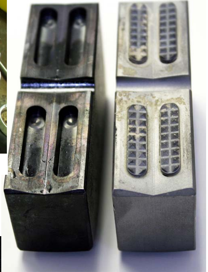
Block before braze (l), flame-processed (r)
