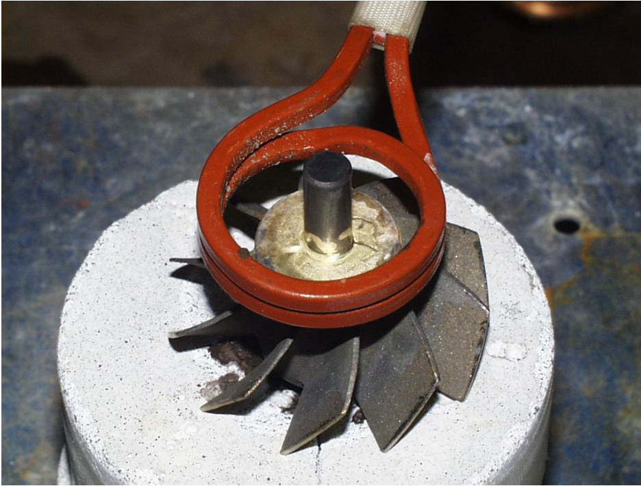
The brazed assembly is shown within the coil
