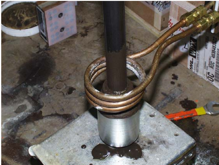
Tube fittings being brazed together via a circular induction heating coil
