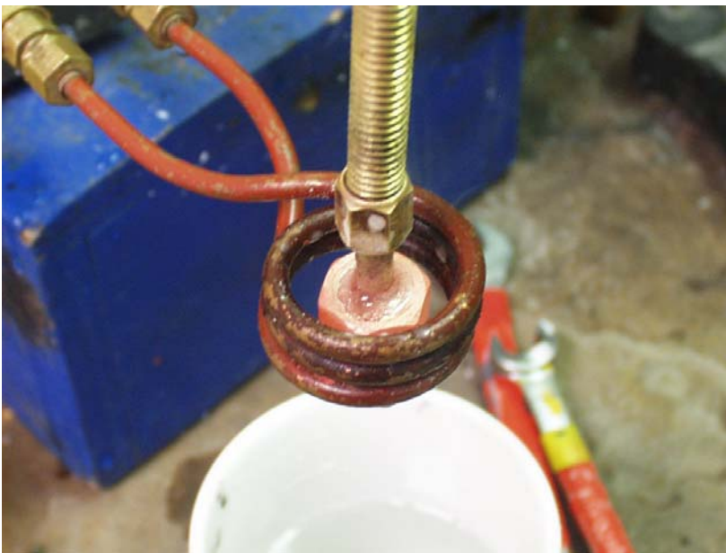
The assembly being heated with the braze flowing
