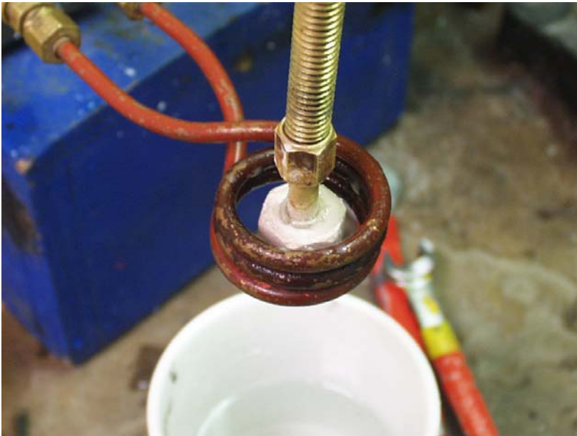
The fluxed steel tube and steel fitting assembly inside the coil
