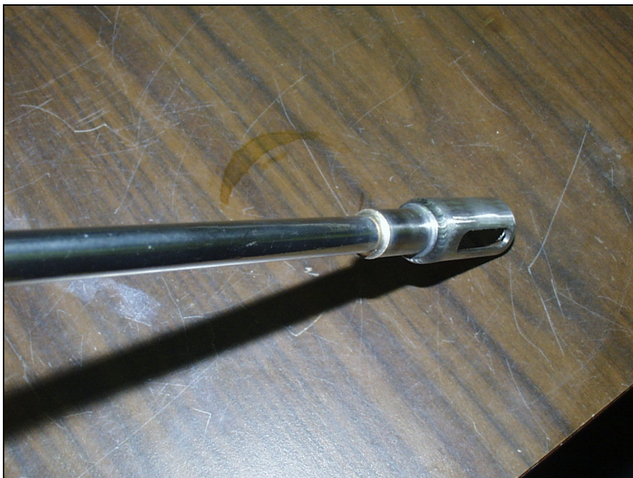
The assembly after brazing.
