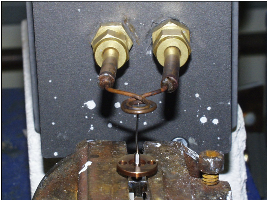
The tungsten carbide ball on top of the steel rod inside a two-turn pancake coil
