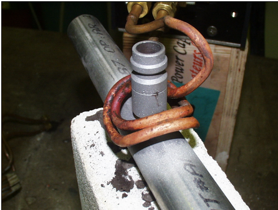
The steel tube and fitting inside the two-turn folded pancake coil (second joint area)
