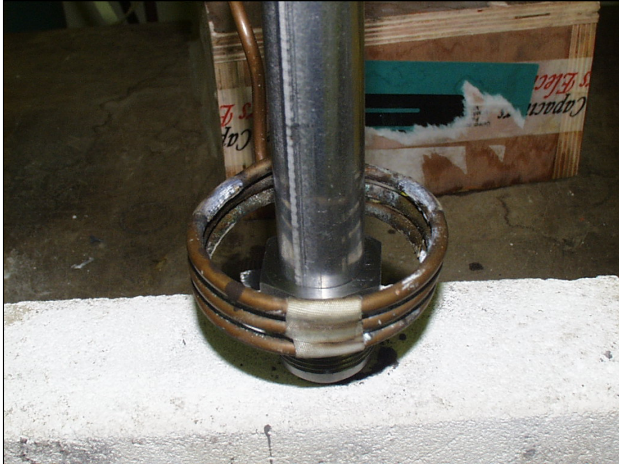
The steel tube and nut inside the three-turn helical coil (first joint area)
