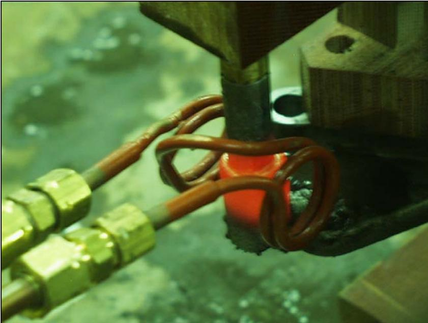
The joint being brazed by a split helical induction heating coil
