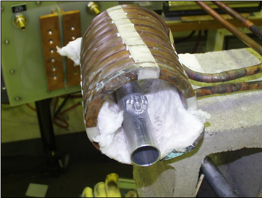
The aluminum assembly inside the induction heating coil
