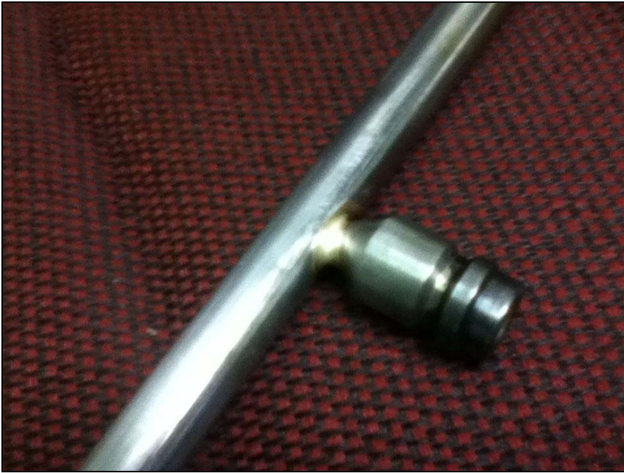
The steel tube and fitting after brazing.
