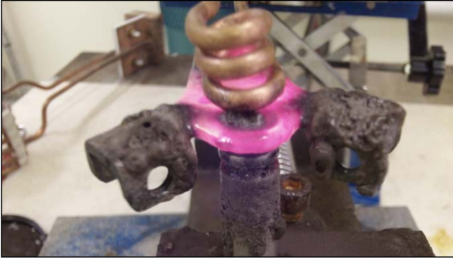
The flange and shaft assembly heating to temperature
