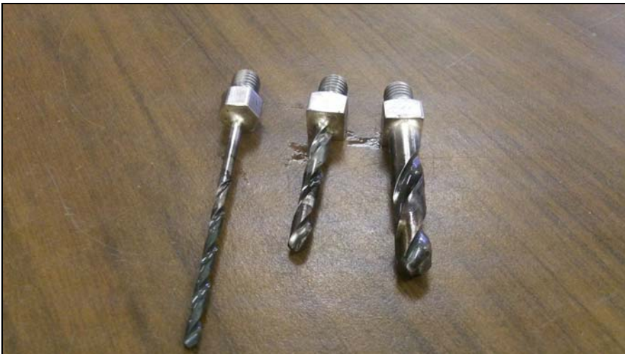
The three steel bits after brazing
