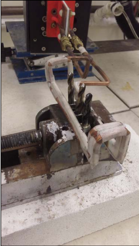
Three steel bits in a channel coil
