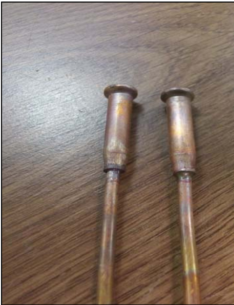
Brazing the copper tubes together
