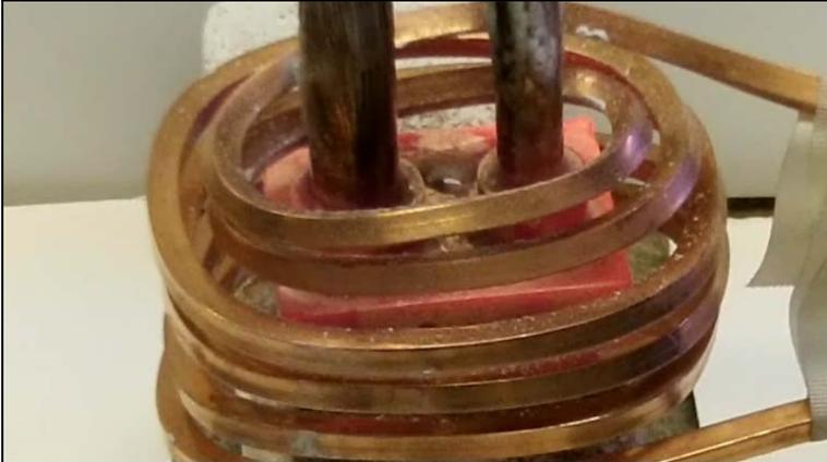
The assembly inside the coil being heated
